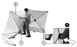
**5.** Firmly hold the two top frame bars with both hands (B) and stand with one foot on the red PVC strips (C) in order to stabilise the lower frame. Now press with either your leg or knee against the fixing disk towards the outside (A), so that the material comes under tension. Conclusion: The four bar ends should be stable before putting the structure under tension.
