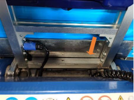
A close-up view of the machine's internal frame. A vertical aluminum carrier is being inserted into a slot. Two orange arrows point to the carrier and the slot, indicating the correct placement. | <p>Führen Sie den vertikalen Träger aus Aluminiumlegierung von CT310 in den entsprechenden Schlitz am Maschinengestell ein.</p> |
