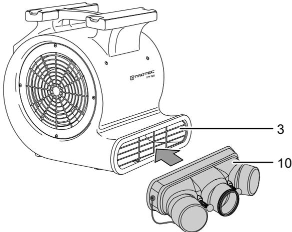
2. Move the attachment hooks (11) around until they are hooked into the air outlet grille (3).
