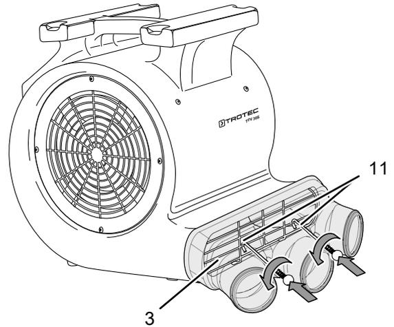
3. Check the three-way hose distributor (10) for tight fit.
